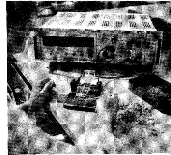
6. Final control of strain gauges, checking the resistance
