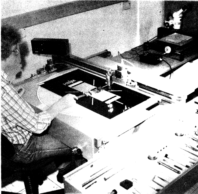
1. Strain gauge master on coordinatograph, prior to reduction
