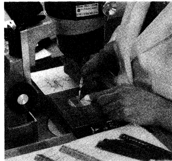
5. Example of further treatment: soldering the ribbons under the microscope
