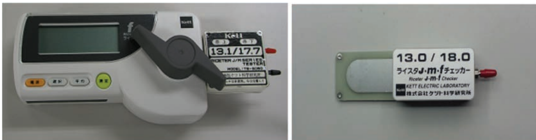
Annex figure 4: Conventional type checker (left) and the latest type checker kit (right)
