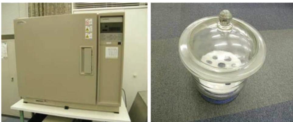
Figure 10: A drying oven (left) and a desiccator (right)
